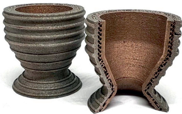
Fig. 3. Multi-material prototypes with lattice elements and tailored properties
