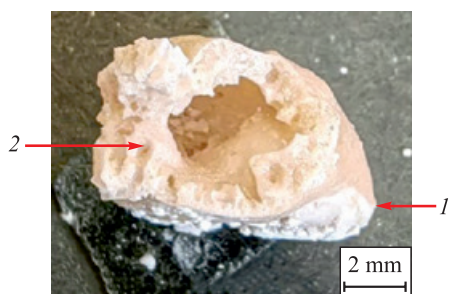
Fig. 2. Photograph of the droplet-shaped (Y_{0.2}Yb_{0.2}Lu_{0.2}Eu_{0.2}Er_{0.2})_3Al_5O_{12} ceramic product (I) showing a cross-sectional fracture (2)
