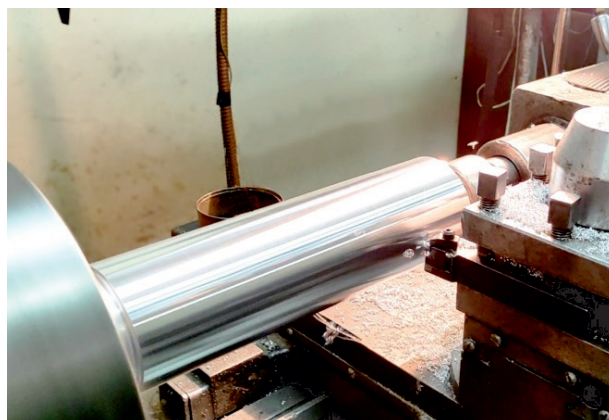
Fig. 2. The machined blank and the cutter during turning
