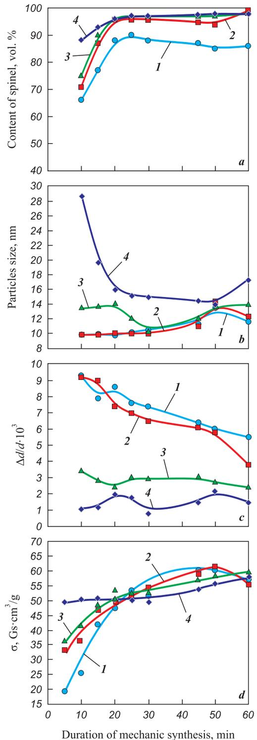
**Fig. 2.** The content of the spinel phase (a), average particle size (b), internal elastic microstresses (c) and saturation magnetization (d) as a function of mechanochemical synthesis time and subsequent heat treatment temperature  $I - t = 20$  °C, 2 – 100 °C, 3 – 300 °C, 4 – 600 °C
