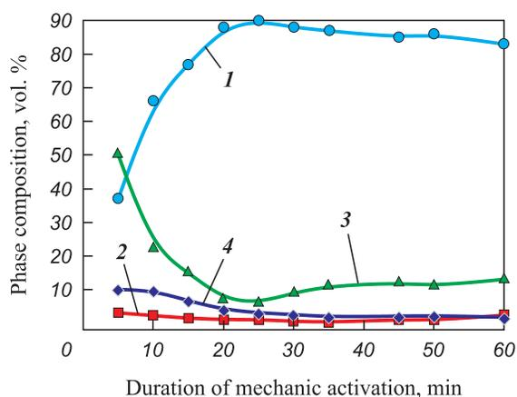
Fig. 1. The phase composition of cobalt ferrosipinel as a function of the duration of mechanochemical synthesis
