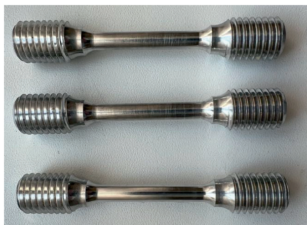
Fig. 7. Samples of dispersed-reinforced MCM for tensile testing
