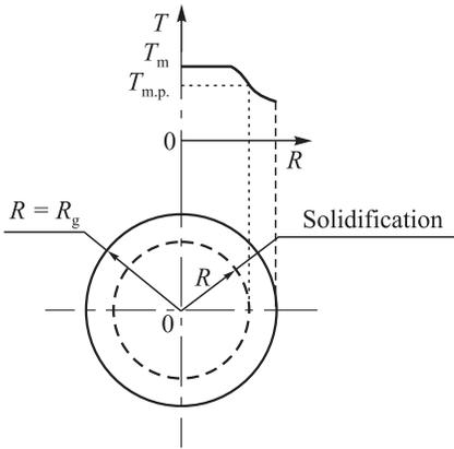
**Fig. 3.** Schematic representation of granule solidification
