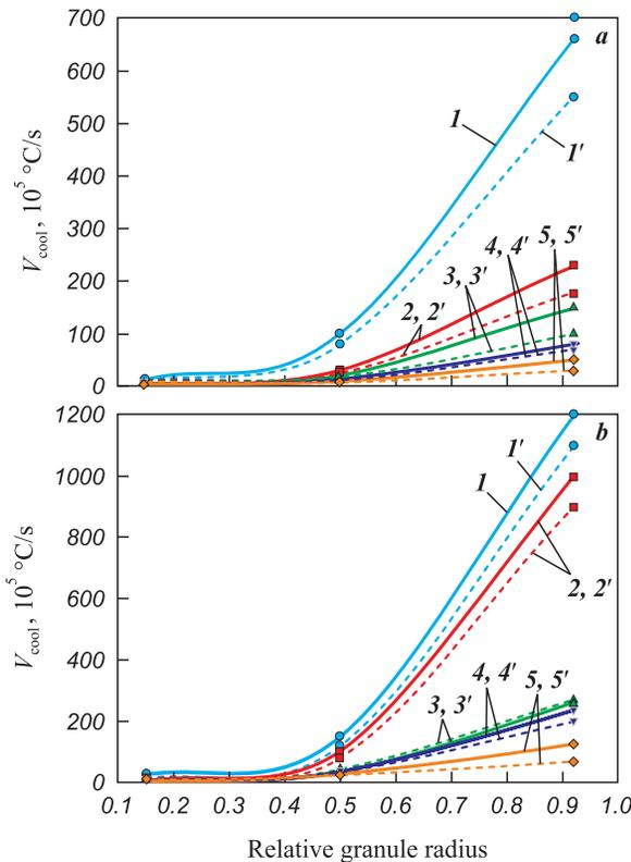
**Fig. 8.** Cooling rate of granules in nitrogen (a) and helium (b), analytically calculated as a function of granule size and gas flow rate
