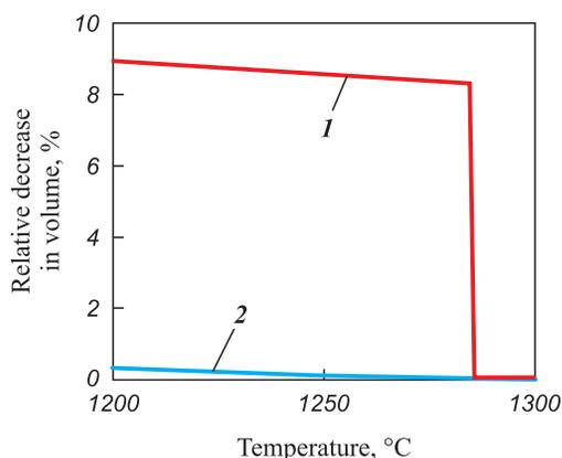
**Fig. 2.** Hypothetical curve of volumetric shrinkage during melt solidification by crystallization (1) and glass transition (amorphization) (2)
