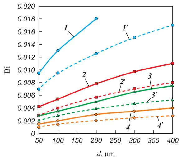
**Fig. 5.** Biot number for gas flow as a function of granule diameter, gas type, and gas flow rate
