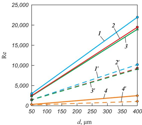
**Fig. 4.** Reynolds criterion for gas flow as a function of granule diameter, gas type, and gas flow rate
