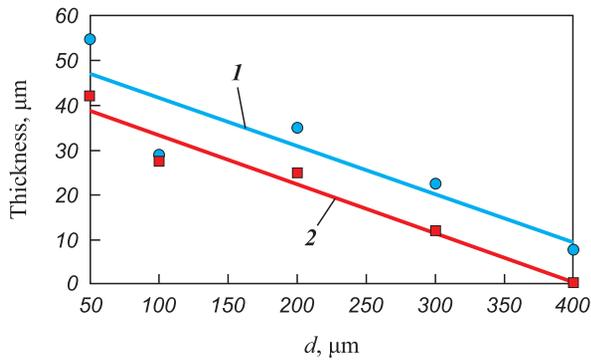
**Fig. 9.** The thickness of the surface shell in relation to the size of beryllium granules and the flow rate of nitrogen (energy-carrying gas)
