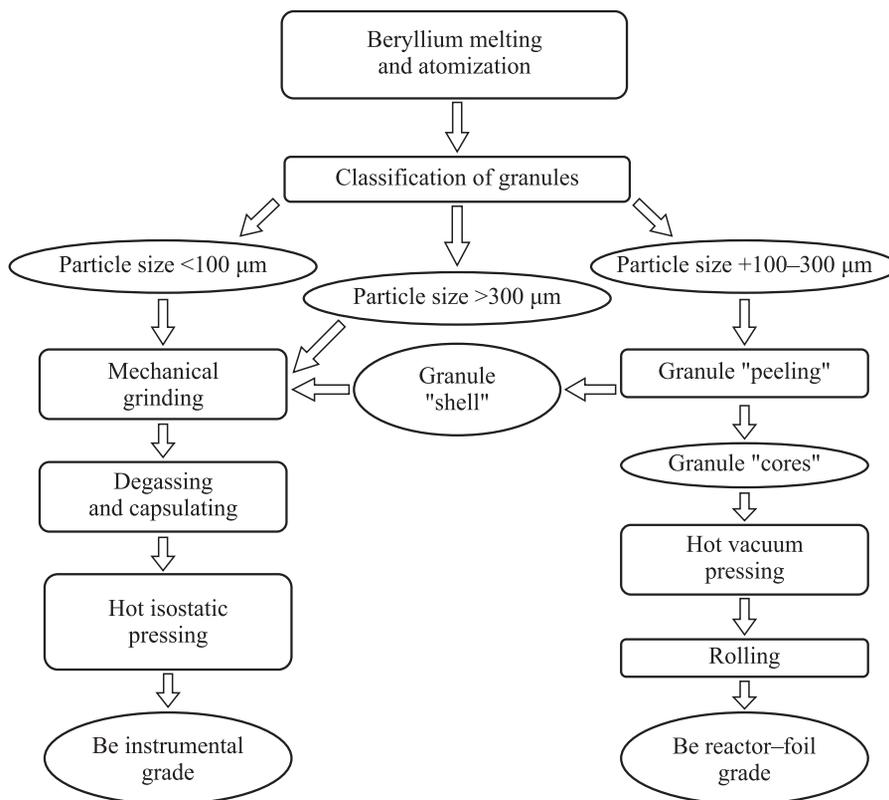
**Fig. 10.** Flowchart of production process for different structural grades of sintered beryllium
