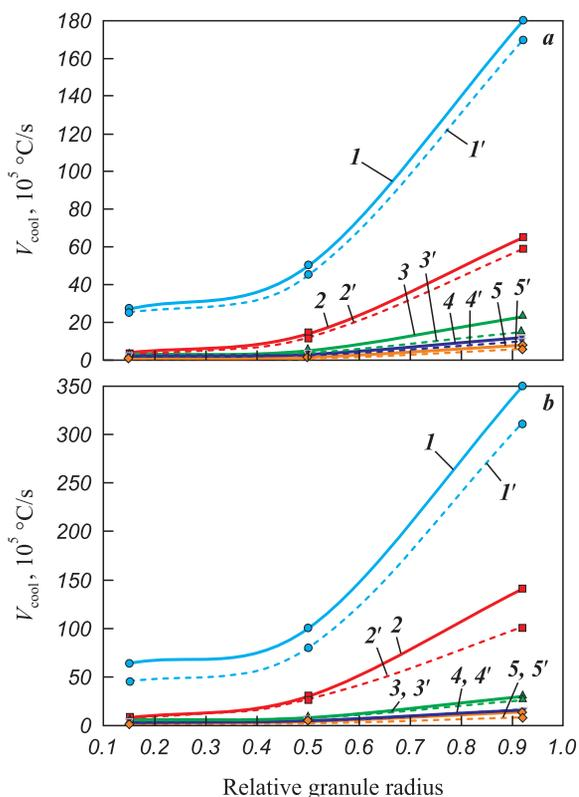
**Fig. 7.** Cooling rate of granules in nitrogen (a) and helium (b), determined through graphical analysis, as a function of granule size and gas flow rate
