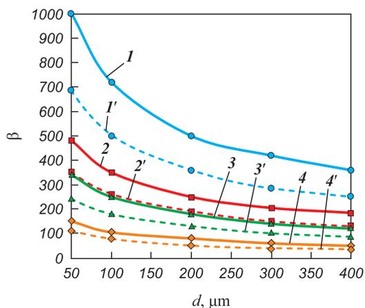
**Fig. 6.**  $\beta = 1/Bi$  as a function of granule diameter, gas type, and gas flow rate
