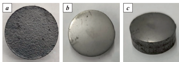
Fig. 3. Photos of (\text{TiZrHfTaNb})\text{C} samples sintered at 2000 °C (20 mm in diameter)
