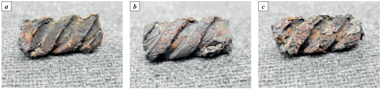
Fig. 8. Matrix samples following sintering in air at t = 900\text{ °C} (a), 1000\text{ °C} (b) and 1100\text{ °C} (c)
