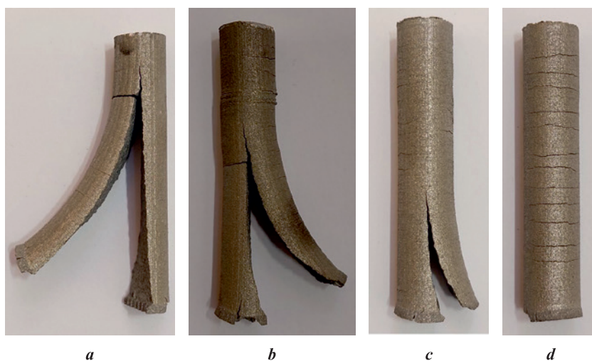
Fig. 4. Samples made from powder 2 a – A1/2, b – A2/2, c – A3/2, d – A4/2
