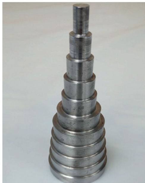
Fig. 2. Cylindrical mandrel with variable diameter
