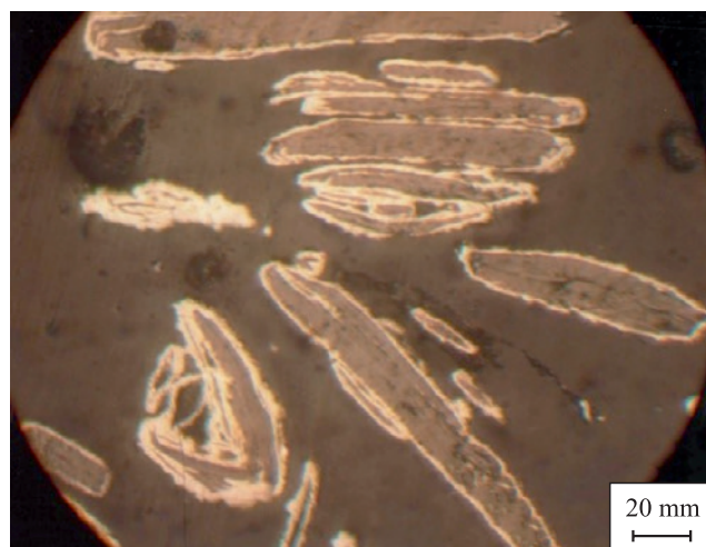
Fig. 1. The structure of the +0.100 mm size particles of the NPG-80 powder
