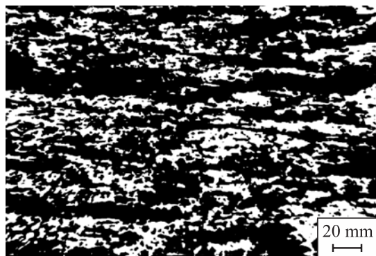
Fig. 4. The microstructure of TSM from NPG-80 powder after electric rolling and subsequent hot rolling White substance – nickel, dark – graphite
