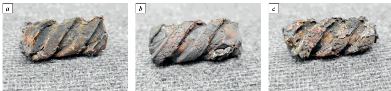
Fig. 8. Matrix samples following sintering in air at t = 900\text{ }^{\circ}\text{C} (a), 1000\text{ }^{\circ}\text{C} (b) and 1100\text{ }^{\circ}\text{C} (c)
