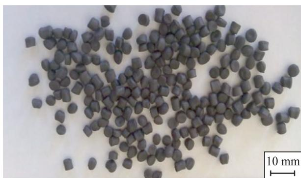
Fig. 2. Appearance of the 09Cr16Ni4Nb feedstock granules
