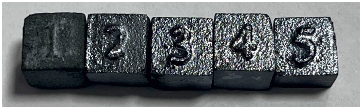
Fig. 4. Cubic specimens – porous SLS SiC preforms after PIP densification and LSI treatment
