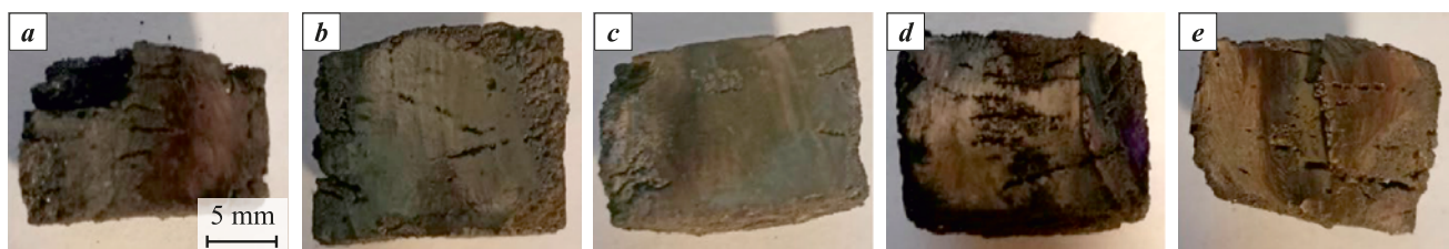
Fig. 4. Macro-images of polished sections of synthesized TiC–Cu cermet samples produced from the SHS charge with 10 % Cu addition at different compaction pressures P , MPa: 22 (a), 34 (b), 45 (c), 56 (d), 69 (e)
